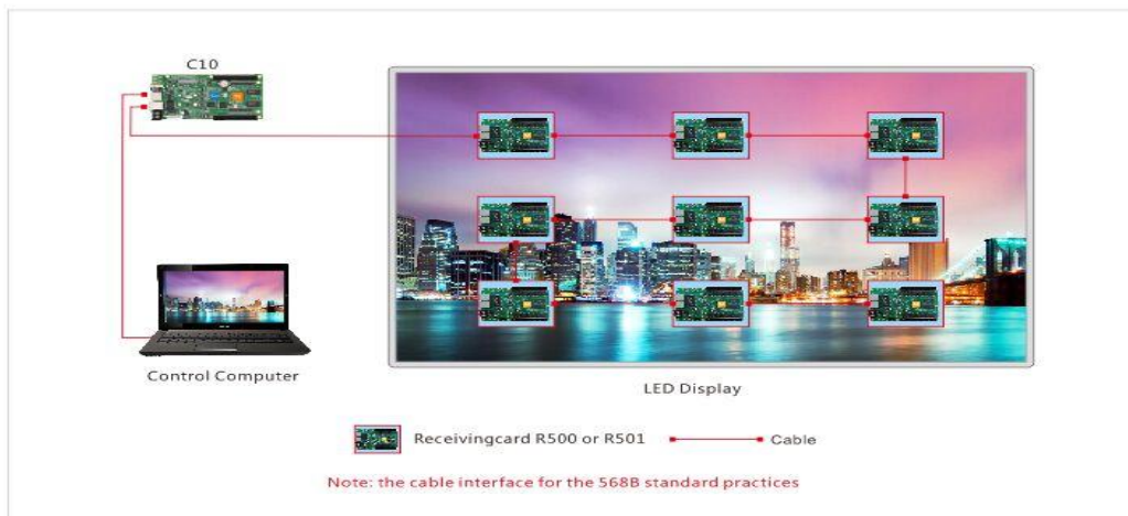
Picture 4-2 only one screen and control by Network cable directly
